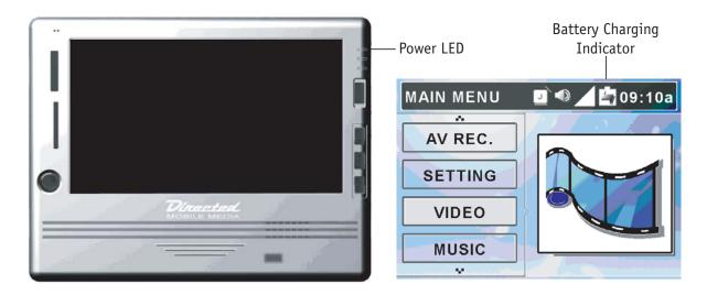
When the battery is fully charged, the Power LED will stop flashing and the charge indicator on the battery icon will disappear. Disconnect the AC Adapter from the player.
